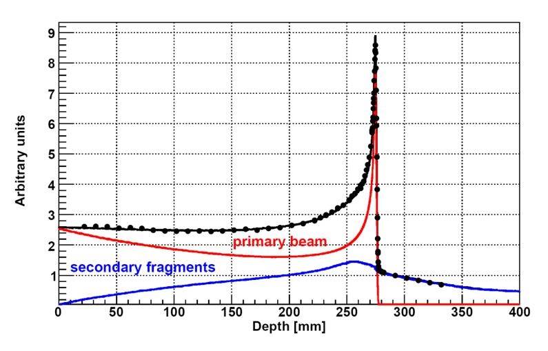
Bragg peak in a water phantom 400 MeV/A C beam: The importance of fragmentation
