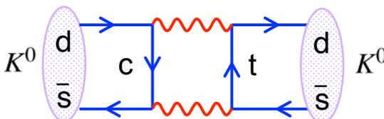
The third term is the 2<sup>nd</sup> order term in the perturbation expansion corresponding to box diagrams resulting in  $K^0 \rightarrow K^0$
